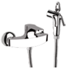
25A/SF Monocomando esterno doccia con doccetta shut-off in ABS cromato, flessibile conico in ottone cromato 120 cm e gancio. Wall mounted single-lever shower mixer with shut-off handshower in c.p. ABS, conical flexible in c.p. brass 120 cm and c.p. hook.
