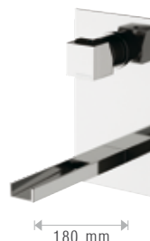
566/RI Miscelatore monocomando a incasso per lavabo, con piastra rettangolare verticale in ottone cromato e bocca quadrata a cascata. Single-lever built-it basin mixer, with vertical rectangular wall flange in chrome plated brass and waterfall squared spout.
