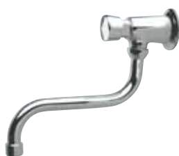
35F/TP Rubinetto frontale temporizzato, con canna "S", 1/2", in ottone cromato, tempo d'apertura 6-8 secondi. Temporized (timer) frontal mounted, with "S" spout, 1/2" tap, all in c.p. brass, opening time 6-8 seconds.
